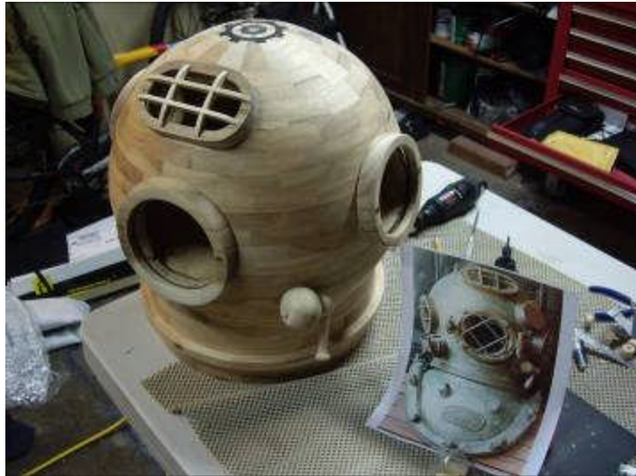
Bill Tarleton showed a 352 piece Segmented Turned Diving Helmet being built as a Hat Box for a US Coast Guard promotion ceremony
