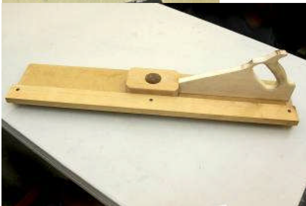
Mike Selser showed a very clever Vacuum Jig for cutting small parts on the Table Saw
